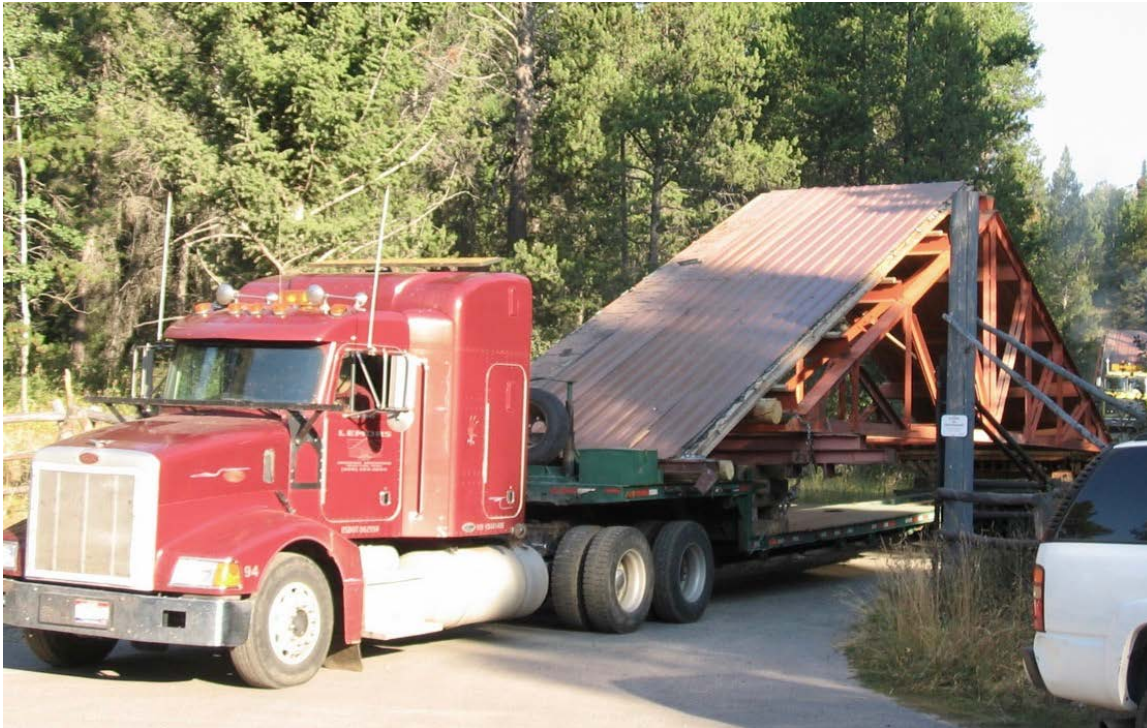
Transporting a 12-foot wide section of the roof to Moose. Photo courtesy of WCHP, 2005.
