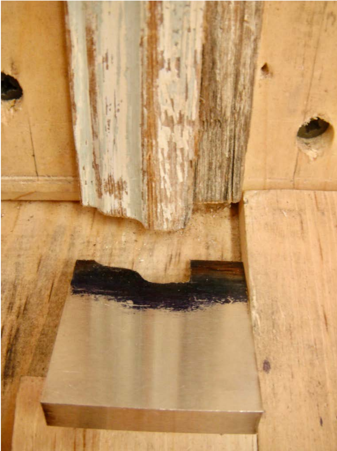
(Top Center) is a wood profile from window that needed to be reproduced, i.e., replicated. (Bottom Center) is a metal knife precision ground to match the profile. A total of three identical knives were created, put on a large shaper machine where wood is run through to create replacement parts matching the original wood profile. Photo courtesy of WCHP, 2014.
